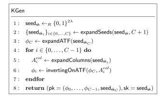
Fig. 1: The pseudo-code for key generation algorithm of ALTEQ.
